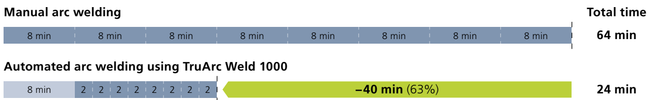
Shipping brace, 8 items with 10 weld seams.
